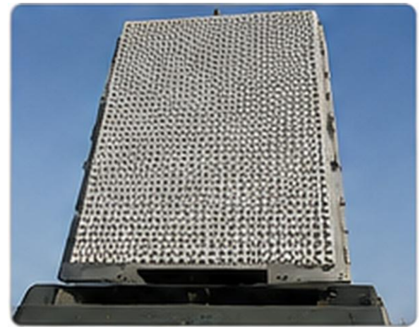
Phased Array Antenna
