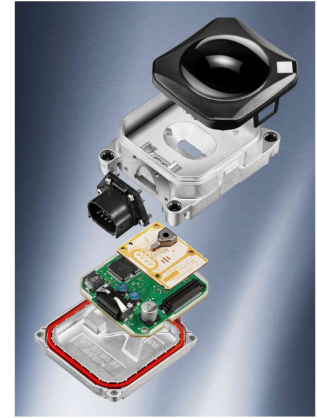
FIGURE 5. Exploded view on the Bosch LRR3 sensor and details of the planar antenna elements feeding the lens. Sensor photograph provided by Bosch.
